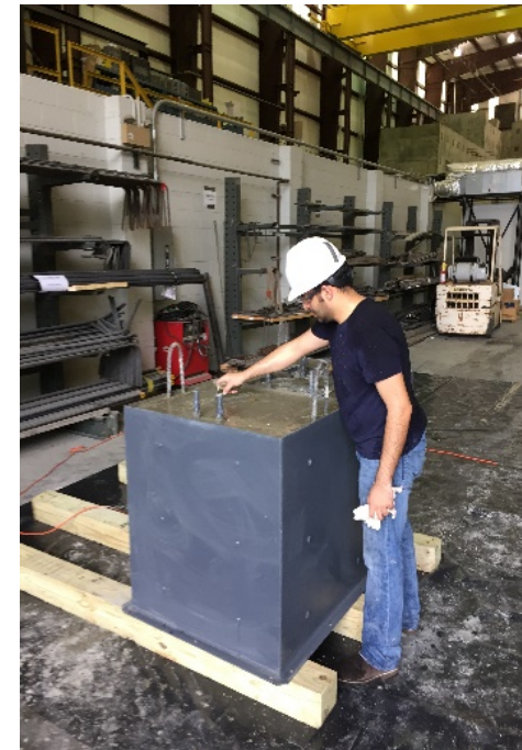
Filling dead mass casing with reinforced concrete
