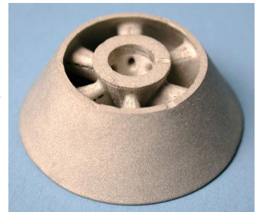
6) Sinter part to produce finished component
