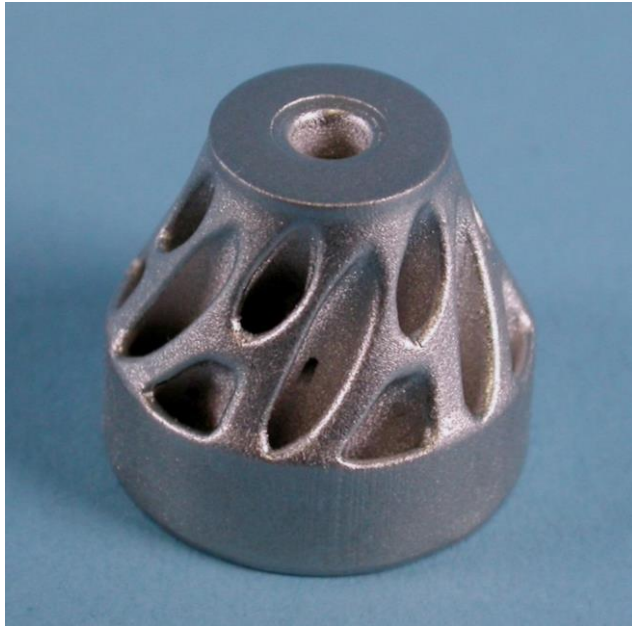
IN 625 nozzle (nickel superalloy)
