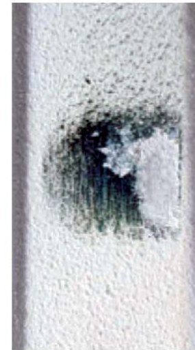
Mixed coating rupture and blade material transfer
