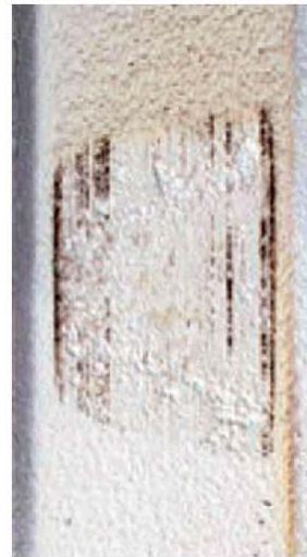
Slight coating rupture mixed with cutting and some blade material transfer
