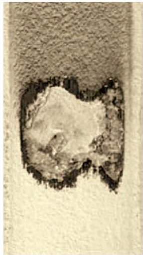
Heavy coating rupture after initial blade material transfer
