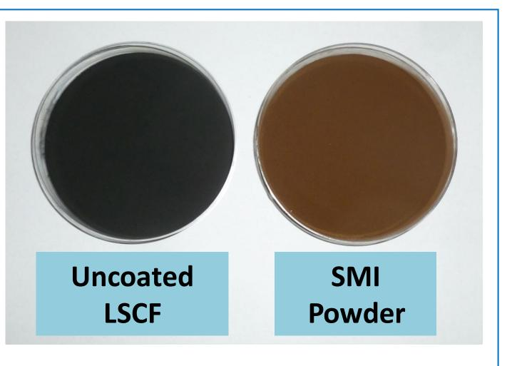
commercial La<sub>0.6</sub>Sr<sub>0.4</sub>Co<sub>0.2</sub>Fe<sub>0.8</sub>O<sub>3- $\delta$ </sub> (LSCF) powder with 0.7  $\mu$ m average particle size, as shown in the image on the left. The image on the right shows a typical powder after surface functionalization by the SMI process.
