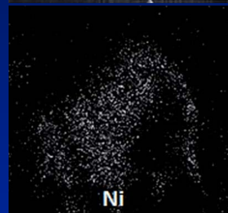
Cross-section and area mapping of an Ni-Fe microparticle after oxidation at 700°C for 30 min
