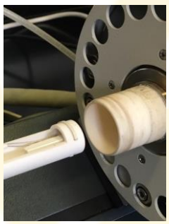
NETZSCH dilatometry setup in WVU for thermomechanical analysis
