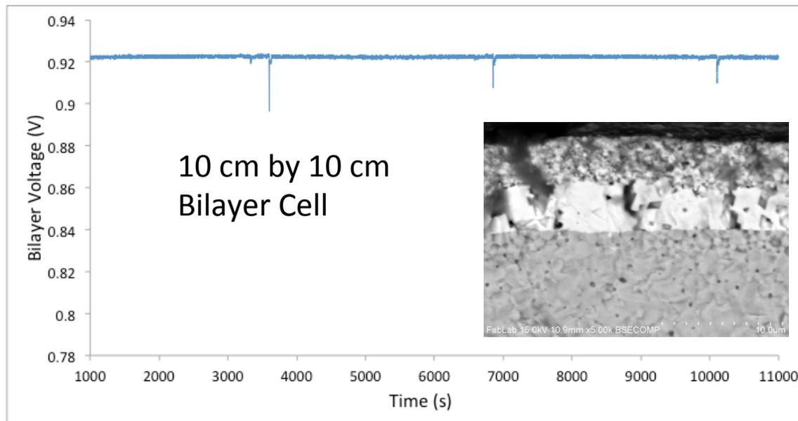
Redox multiphysics model showed that closed & open pores can reduce OCV due to ineffective TBP and decreased conductivity (leakage current in GDC)
