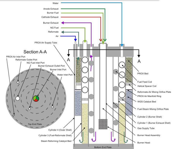
Figure 15: Reactor Diagram
