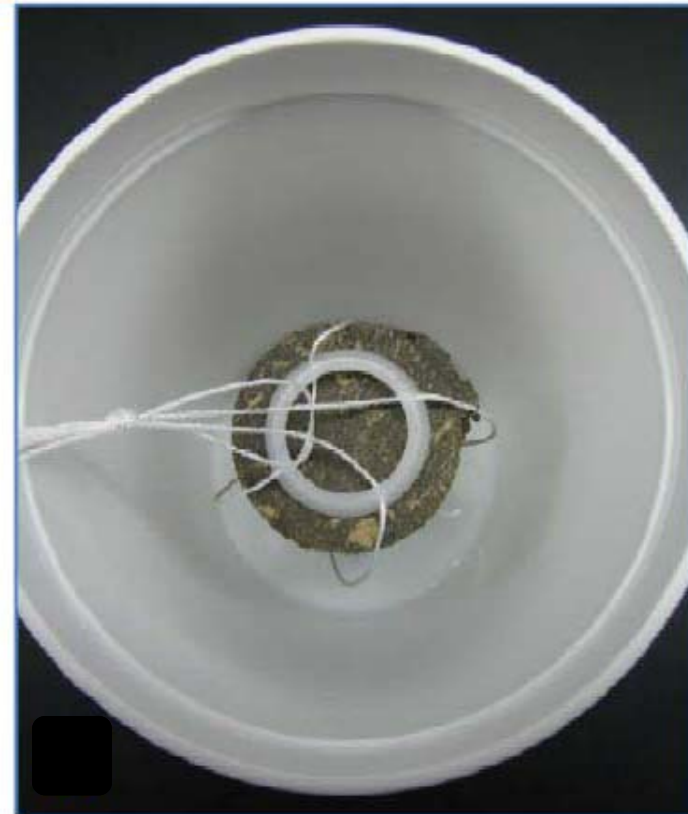
Sample Centered in Eluant (top view)
