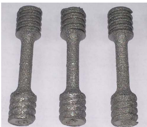
Fabricated tensile dog-bone samples
