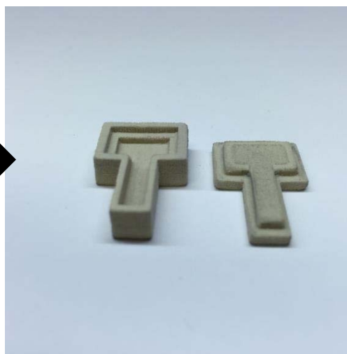
Sintered at 1600°C for 16hrs
