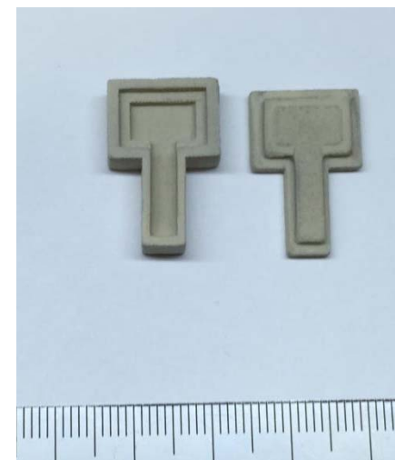
Sintered at 1600°C for 16hrs
