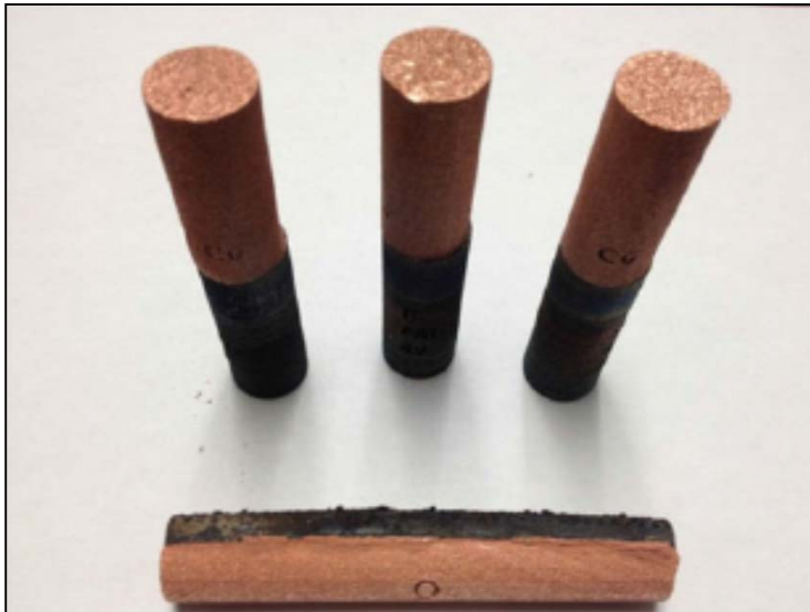
Multi-material fabrication using EBM [1]
