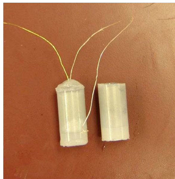
Schematic design and image of the downhole CO 2 sensor.
