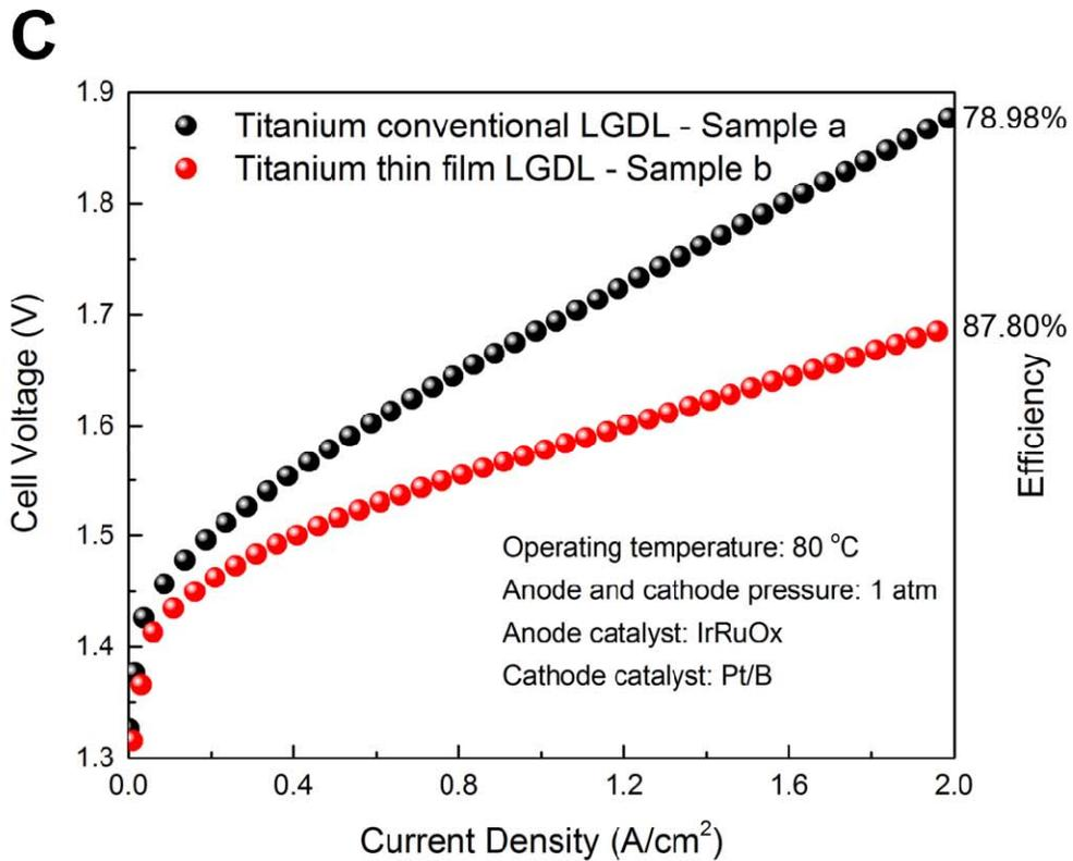
Efficiency improved from **78% to 87%** at a current density of 2.0 A/cm<sup>2</sup>
