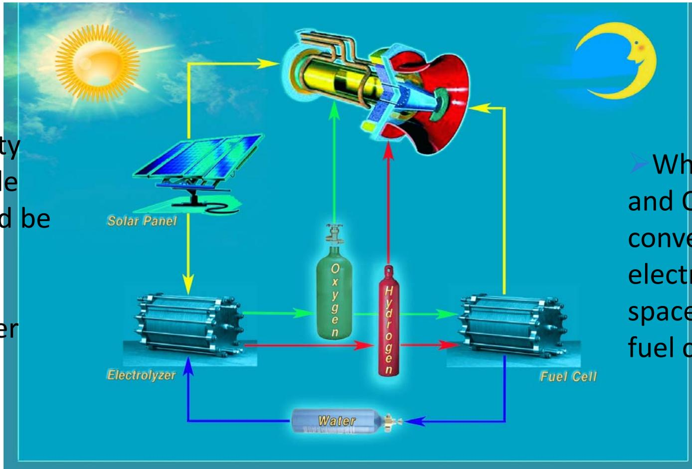
➤ When needed,  $H_2$  and  $O_2$  will be converted back to electricity to power space craft via micro fuel cells
