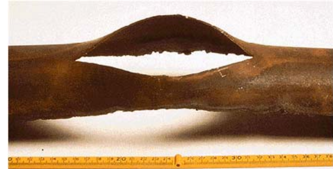
ruptured steel boiler pipe http://sirius.mtm.kuleuven.be/
