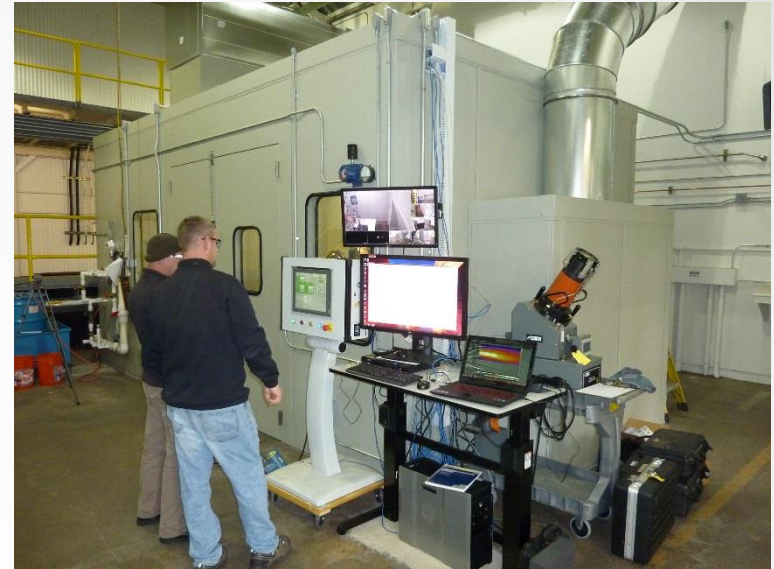
“remote” MHD testing inside a 20' x 12' booth
