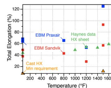
Similar tensile properties for the two EBM HX alloys
