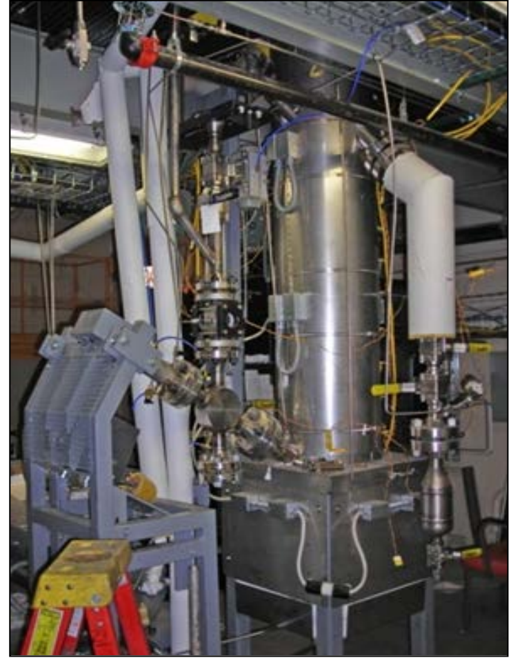
Fluid-Bed Gasifier (FBG) 800°C, 600 psi
