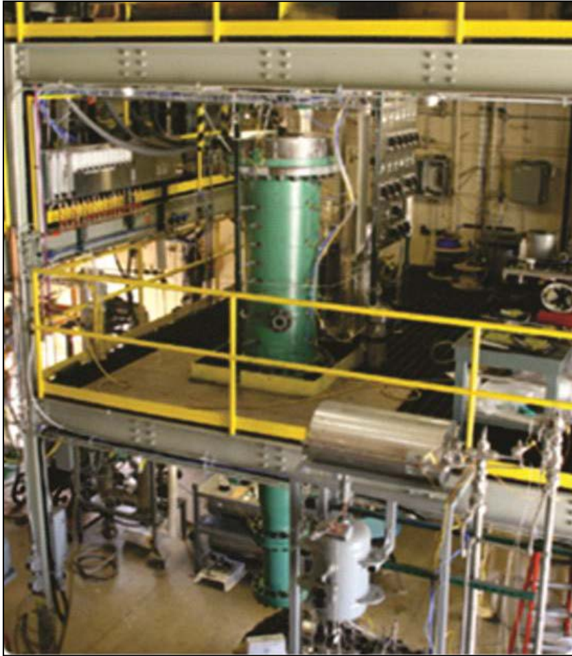
Entrained-Flow Gasifier (EFG) 1800°C, 300 psi
