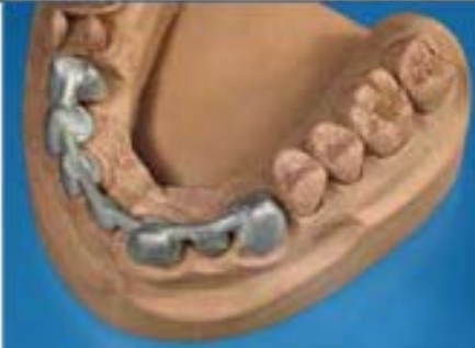
Powdered material is solidified into a cross-section of a model with laser
