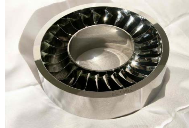
Flow Straightener for Helicopter Engine (Killian 2013)
