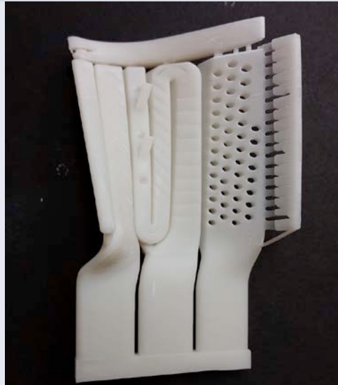
LAMP-Manufactured Generic Aviation Airfoil Core and Integral-Cored Shell Mold
