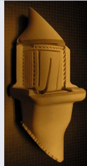
LAMP-Manufactured Generic Aviation Airfoil Core and Integral-Cored Shell Mold
