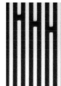
250 MHz: fingerwidth 3 \mu\text{m}
