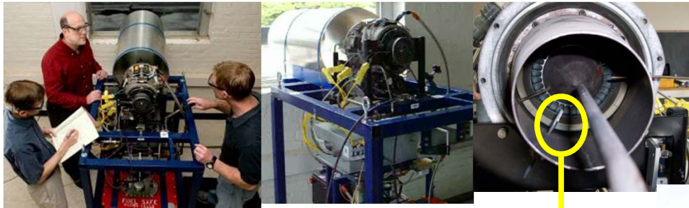
SAW sensors mounted on probes inserted into engine exhaust
