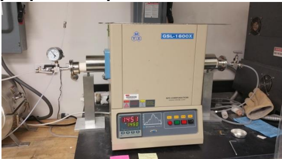
Furnace for measuring electrical properties up to 1500 °C
