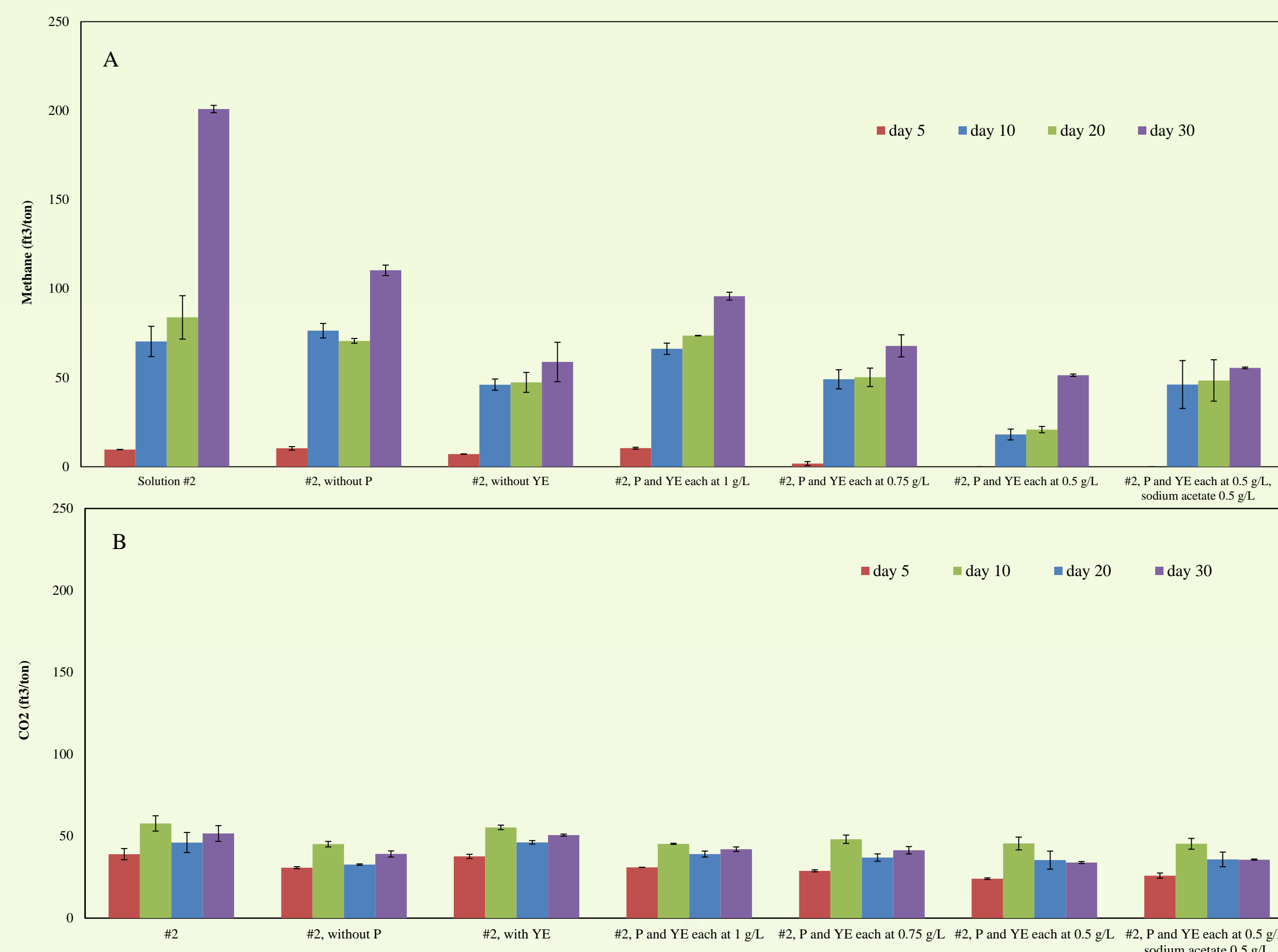
Fig. 4: Yield of gas on bituminous coal under different conditions. A: Methane, B: CO 2 .
