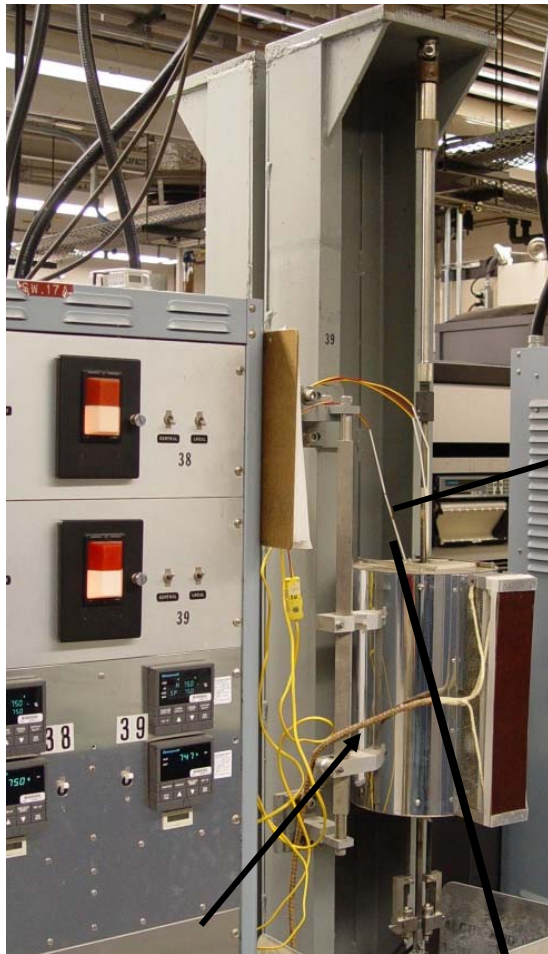
LVDTs for Continuous Monitoring of Creep Strain
