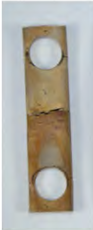
Grade 315 Jones and C-ring test specimens in aerated H 2 O, 200°C, 168h
