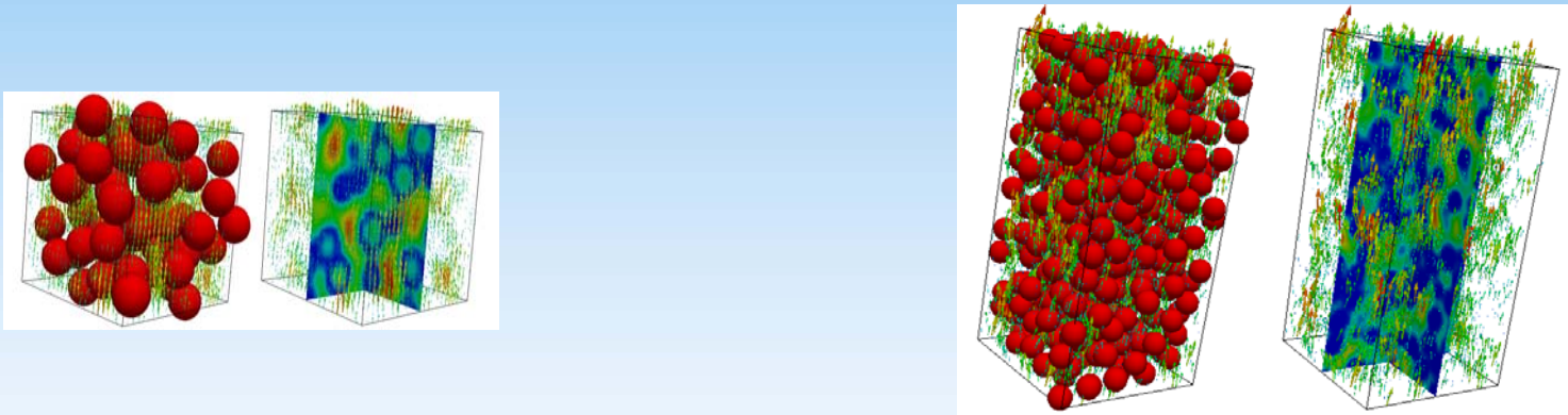
LEFT: Flow over a random distributed 60 spheres; RIGHT: Flow over 405 spheres. The same pressure gradients are applied. Solid volume fraction for both cases: \phi=0.345 .
