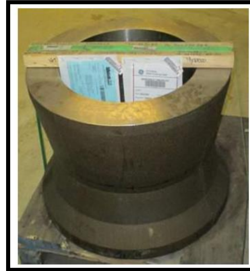
Haynes 282 centrifugal casting: 635kg (1,400lbs)
