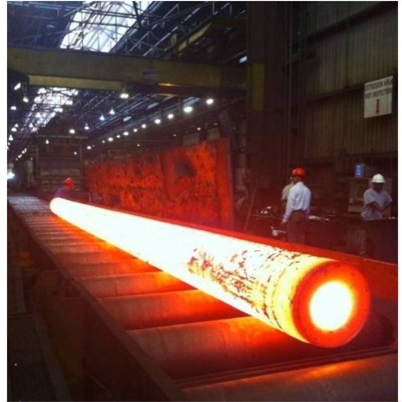
Inconel®740H Pipe after Extrusion at Wyman-Gordon
