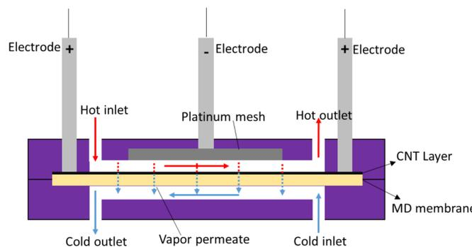
Schematic representation of the ECMD test cell, electrodes, and CNT modified MD membrane. Arrows indicate flow direction of the hot/cold streams. Dotted arrows represent vapor flux across MD membrane.
