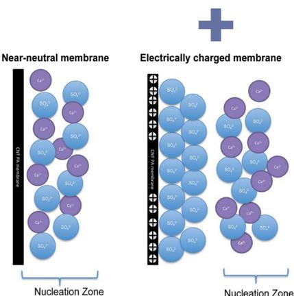
**Charged membrane surface alters the mechanism by which scale is formed**
