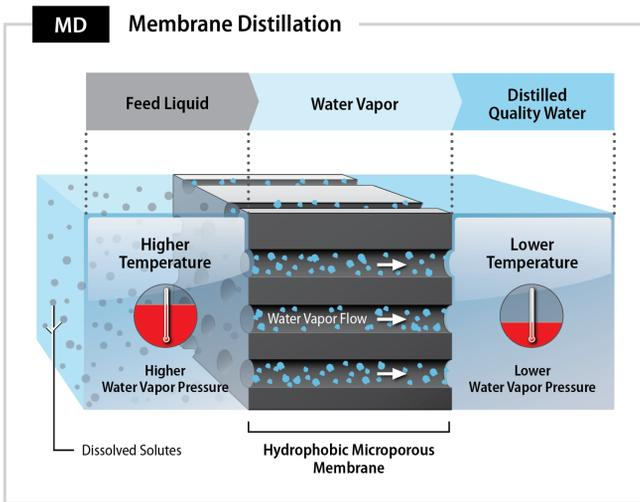
Illustration showing the MD process. The hydrophobic membrane facilitates vapor transport via a temperature differential.
