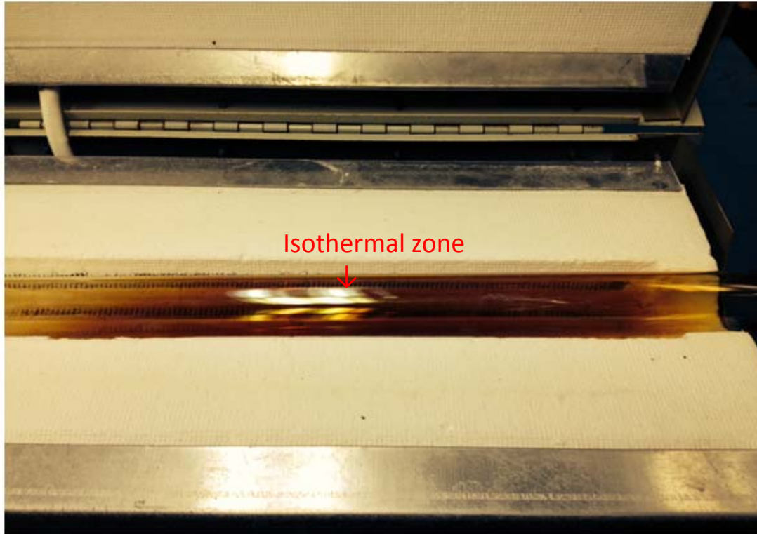
AP-MOCVD hot wall reactor with deposited iron oxide at 220°C
