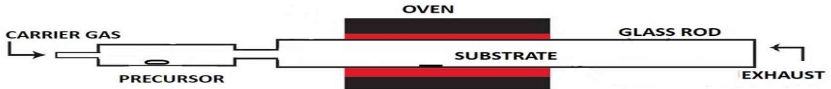
Schematic illustration of a horizontal CVD hot-wall reactor
