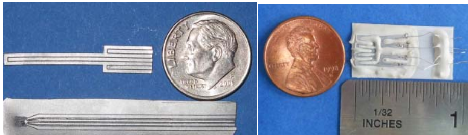
Sintered Structures and Packaged MoSi 2 Sensor Element
