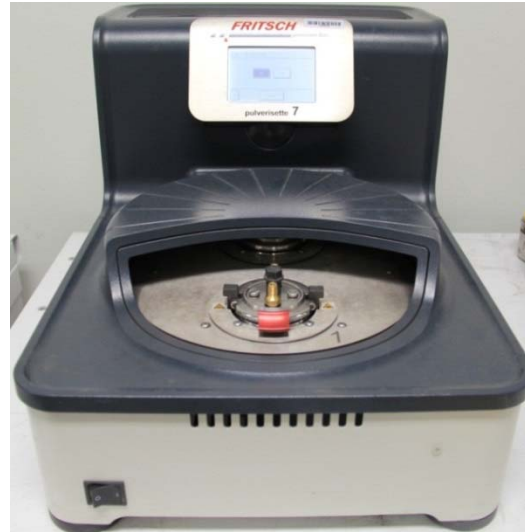
Planetary ball mill (Fritsch Pulverisette 7)
