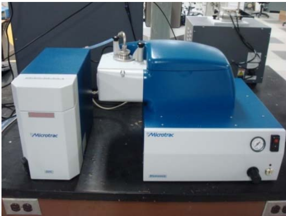
Particle size analyzer (Microtrac Bluewave)
