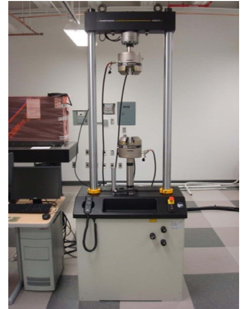
Fatigue test machine (Instron 8801)
