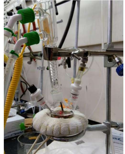
Bubble reactor for catalysts screening tests
