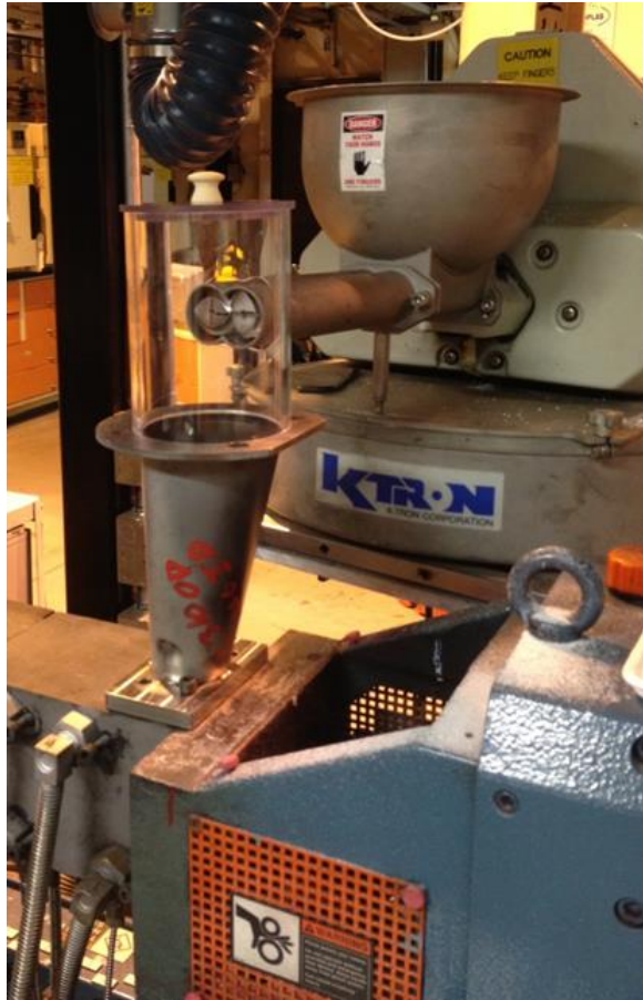
K-Tron solids feeder and 25mm extruder, connected to desorber inlet
