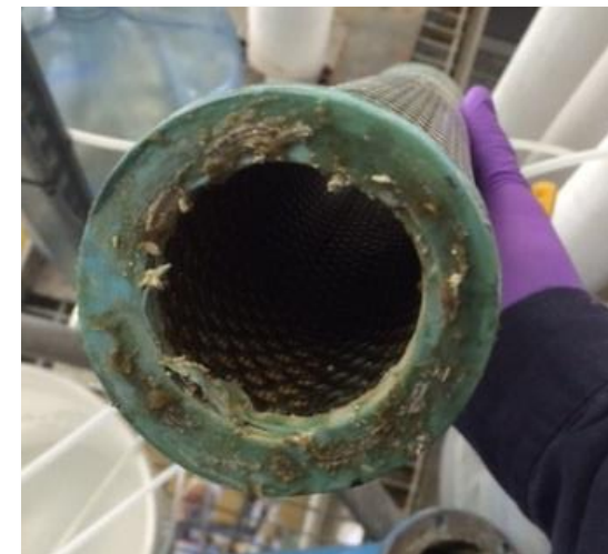
Fouling of bench system filters
