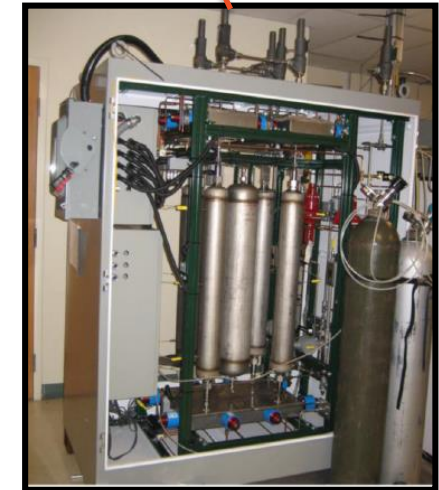
TDA Shift/Separation Skid
