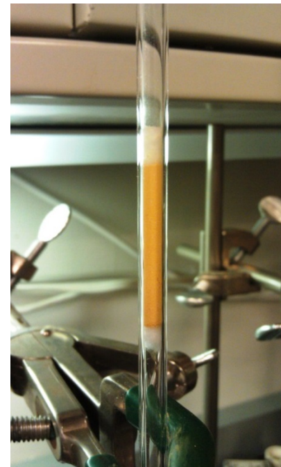
Batch mode reactor for catalyst evaluation.
