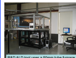
R&D ALD tool uses a 50mm tube furnace
