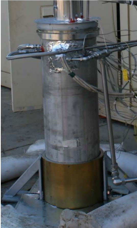
Well head suspending the stack modules from the surface
