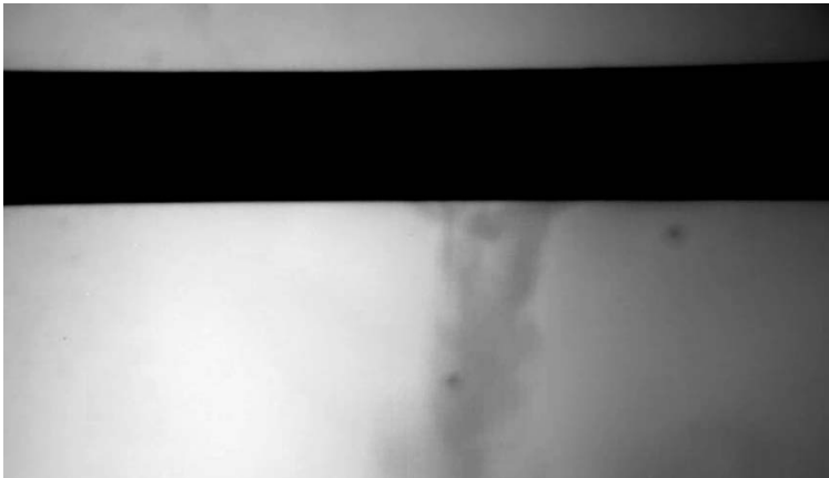
Crack visualization by IR absorption of CO 2
