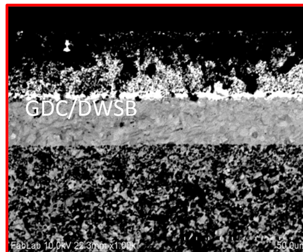
M1.1.2: Demo button cell with optimized relative/total bilayer thickness for OCP~1V
