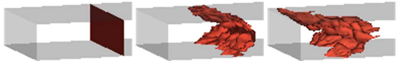
Flame Flashback in Confined Geometries
