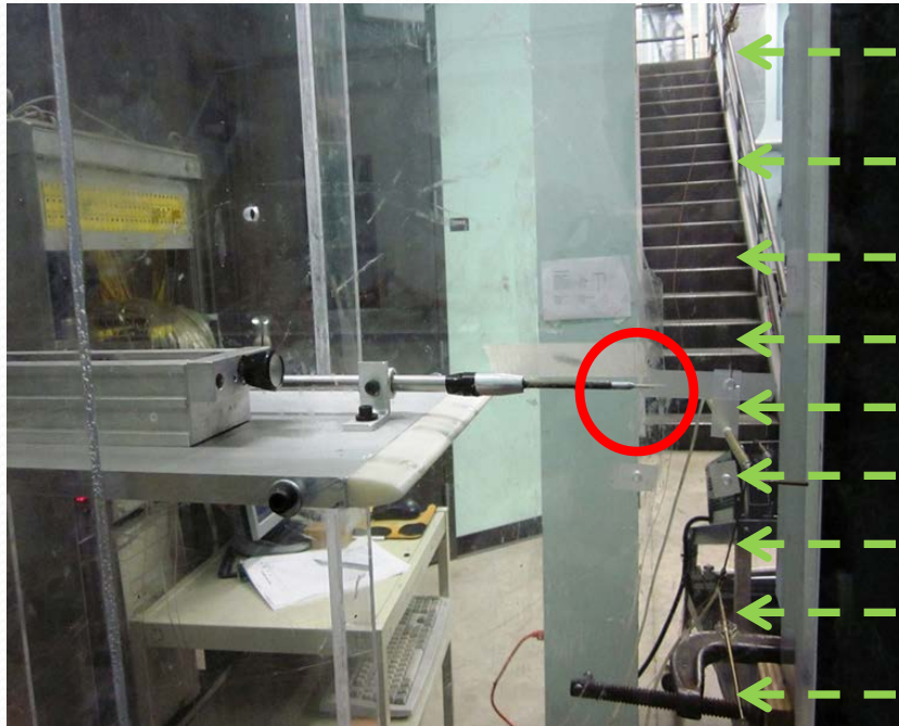
Turbulence decay measurements began without the cylinder in place.
