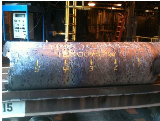
VAR Ingot: 24in Diameter x 71in long, ~10,000lb
