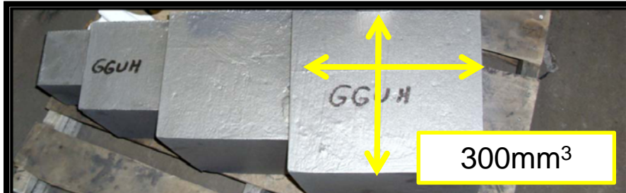
Haynes 282 and Alloy 263 Step Castings 135-450kg sizes (300 to 1,000 lbs)
