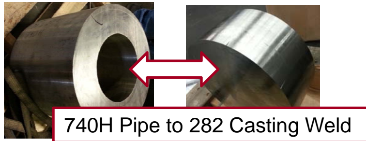
Simulated casting weld defect repair
