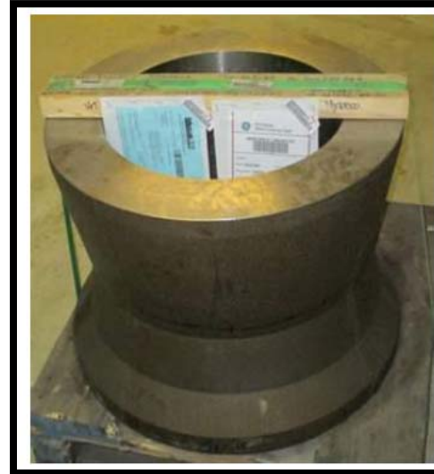
Haynes 282 centrifugal casting: 635kg (1,400lbs)
