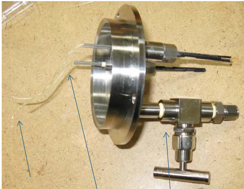
Flange with Pt Wire Connection Up to 8 total connections
