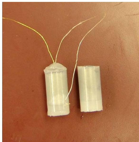
Figure. 29 Schematic design and image of the downhole CO 2 sensor.
