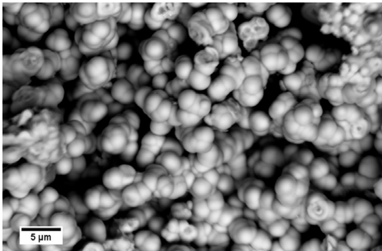
Plan view SEM image of Mo particles on Nb sample
