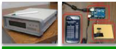
Electric grid frequency monitoring network (FNET / GridEye)
