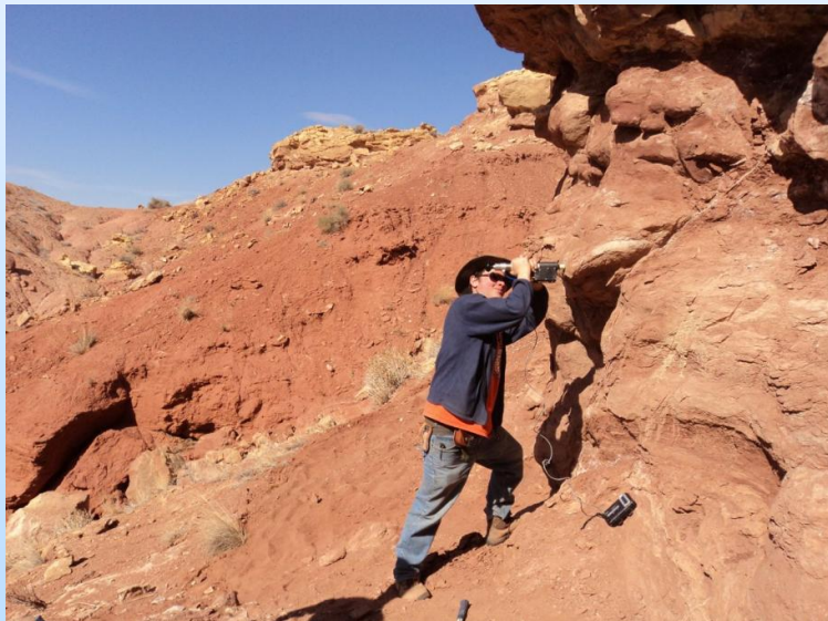
Outcrop permeability measurements using TinyPerm™
