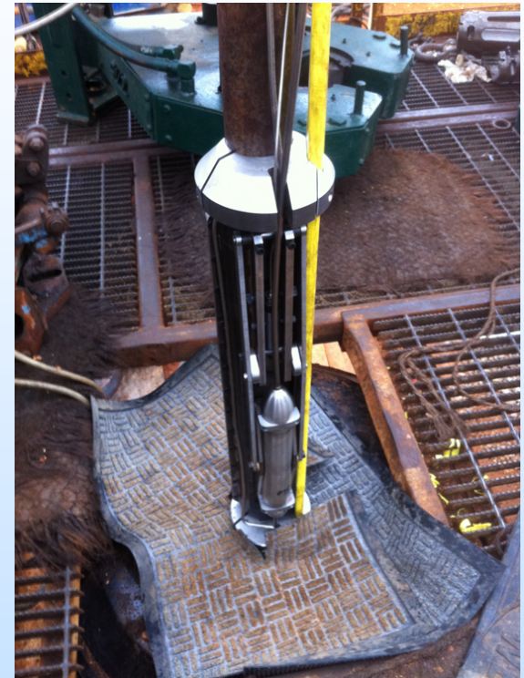
Geophone pod and clamping assembly and yellow flat pack containing fiber cable
