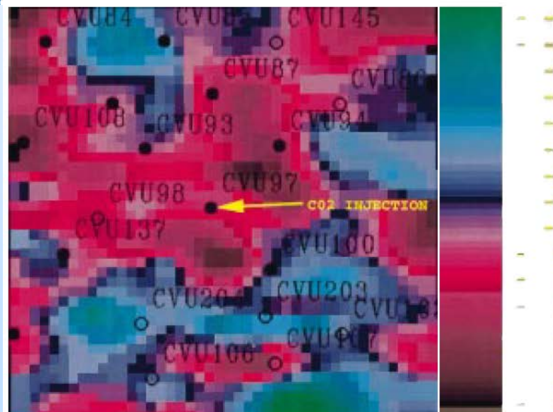
Figure 6. Velocity anisotropy map from the repeat 3-D, 3-C survey. The zone of zero percent anisotropy from the base survey is now showing 6% positive anisotropy, indicating a higher density of vertical open fractures parallel to the maximum horizontal stress direction or stiffening of the frame due to viscosity and/or saturation change of the fluid and a reduction in bulk density.
