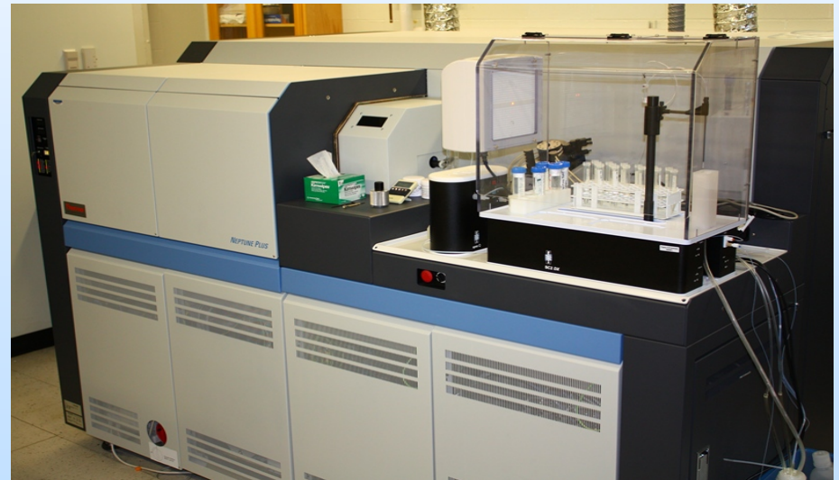
NETL's Thermo Scientific NEPTUNE PLUS MC-ICP-MS at the University of Pittsburgh, Dept. of Geology and Planetary Science.
